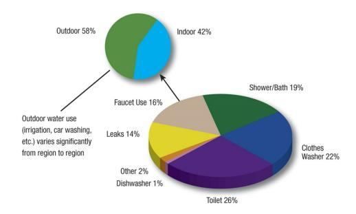
Typical Western Water Use: Non-Potable water supply development significantly reduces overall irrigation demand and removes +/- 60% potable demand from residential supply
